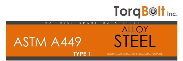
ASTM A449 covers headed bolts, rods, and anchor bolts in diameters ranging from 1/4" through 3" inclusive. It is a medium strength bolt manufactured from a medium carbon or alloy steel that develops its mechanical values through a heat treating process. It is intended for general engineering applications.
