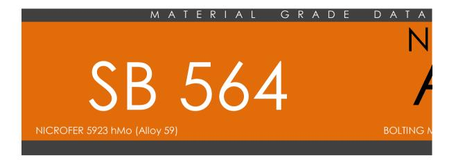
SB 564 covers nickel alloy forgings. These alloys are classified into different grades according to their chemployed on each alloy in order to determine its chemical composition. Grain size and mechanical pelongation shall be measured. A tension test and nondestructive ultrasonic test shall be done on each alloy UNS N06059. The values stated in inch-pound units are to be regarded as standard. The values gives to SI units that are provided for information only and are not considered standard.
