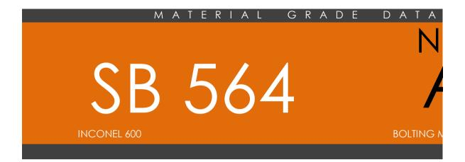
SB 564 covers nickel alloy forgings. These alloys are classified into different grades according to their ch employed on each alloy in order to determine its chemical composition. Grain size and mechanical p elongation shall be measured. A tension test and nondestructive ultrasonic test shall be done on each N06600. The values stated in inch-pound units are to be regarded as standard. The values given in pare that are provided for information only and are not considered standard.
