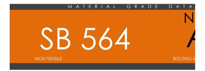
SB 564 covers nickel alloy forgings. These alloys are classified into different grades according to their chemployed on each alloy in order to determine its chemical composition. Grain size and mechanical pelongation shall be measured. A tension test and nondestructive ultrasonic test shall be done on each alloy UNS N06686. The values stated in inch-pound units are to be regarded as standard. The values giv to SI units that are provided for information only and are not considered standard.
