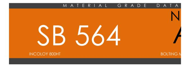
SB 564 covers nickel alloy forgings. These alloys are classified into different grades according to their chemployed on each alloy in order to determine its chemical composition. Grain size and mechanical pelongation shall be measured. A tension test and nondestructive ultrasonic test shall be done on each N08811. The values stated in inch-pound units are to be regarded as standard. The values given in pare that are provided for information only and are not considered standard.
