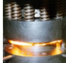
Heading press is engaged and punches down & forms Head
